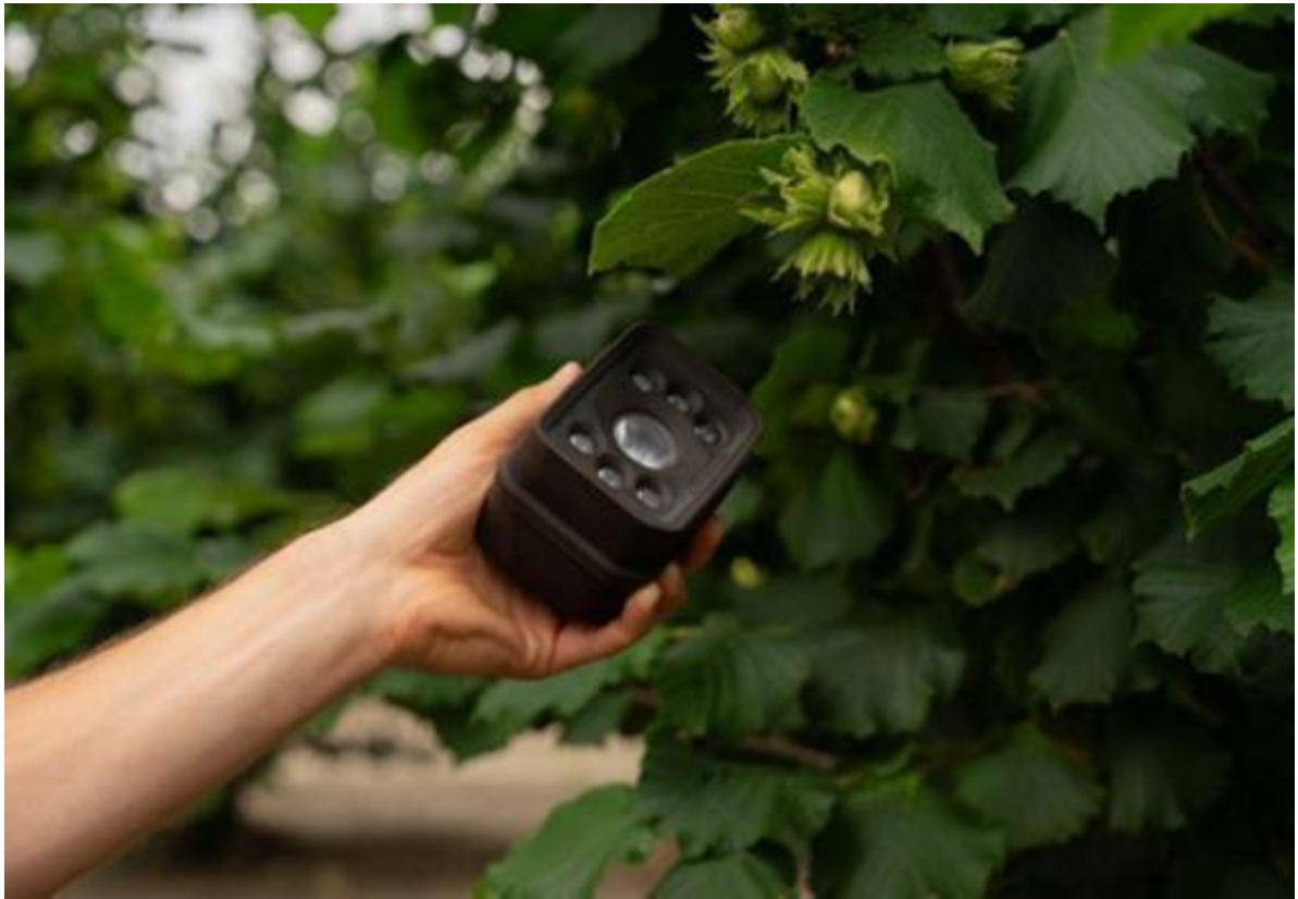
Figure 3 Plant-O-Meter - a crop monitoring device developed by the BioSense Institute.
